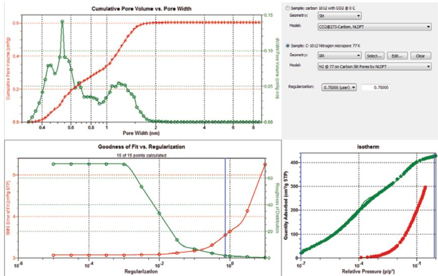
This advanced NLDFT method allows users to determine the pore size distribution of their sample using two isotherms. In this example CO<sub>2</sub> adsorption (red) at 273 K and nitrogen adsorption (green) at 77 K are used to calculate a single pore size distribution. Users do not have to cut and paste distributions from CO<sub>2</sub> and nitrogen - a single distribution is determined using both isotherms.
